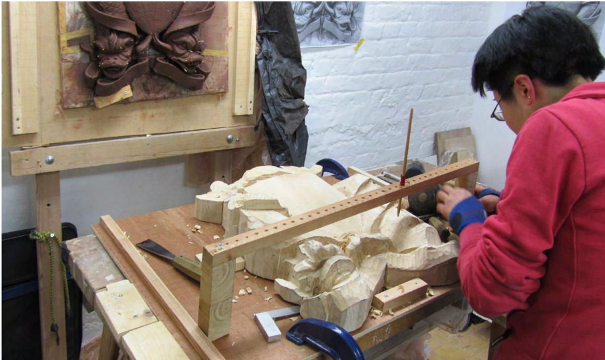
A simple Pointing Machine in operation © Ingalv Maxwell
