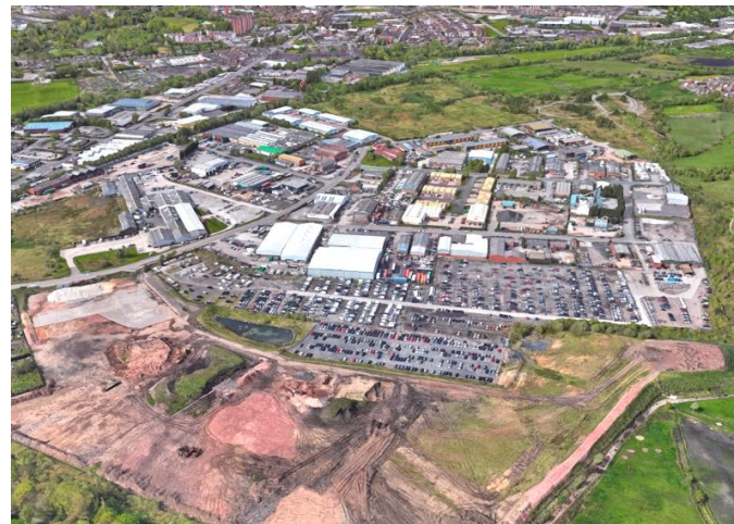
Fig.4.10 Berry Hill Industrial site in 2003, in a similar view from the south-east illustrating the significant degree of back-filling of the former marl pit © Google Earth
