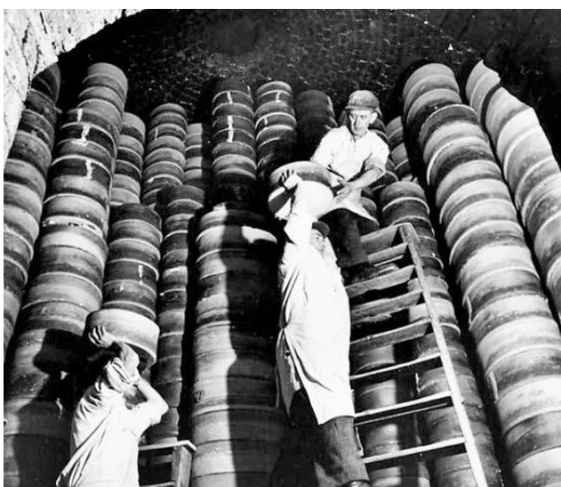
Fig.3.16 Saggar placement in a firing chamber.
