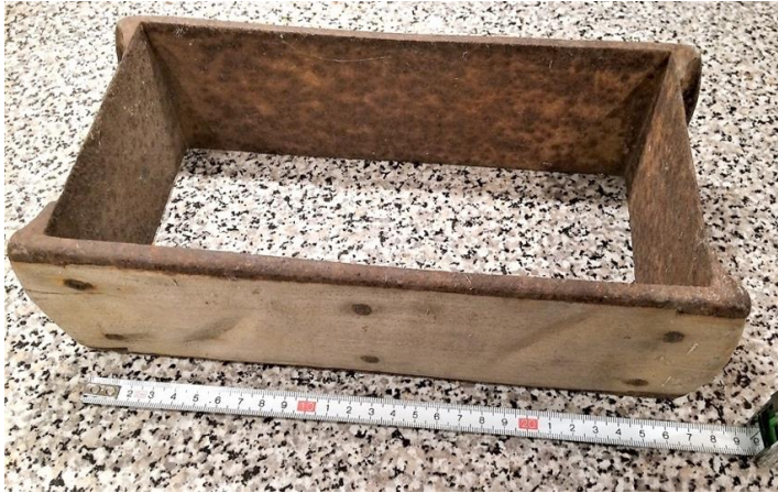
Fig.3.11 Hand-made brick-making mould, metal lined for durability in use. The internal dimensions are oversized to allow for shrinkage when drying and firing *
