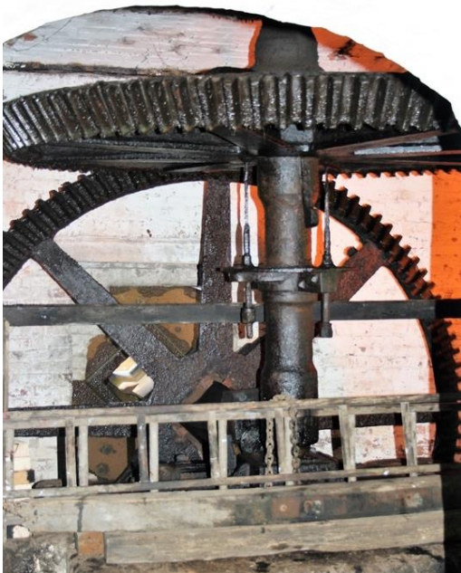
Fig.8.8 Cheddleton cast iron internal bevelled drive gear *
