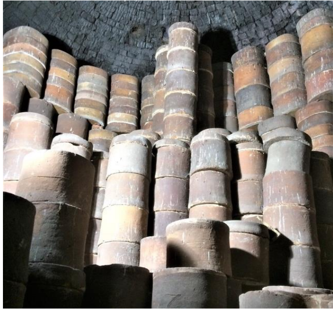
Fig.2.30 Inside an inner firing chamber with saggars stacked ready for firing. The inner chamber of updraught and downdraught kilns had domed floors over the underlying flues. External horizontal iron bands or Bonts reinforced the inner chamber to cope with high temperature variations during firing and cooling *
