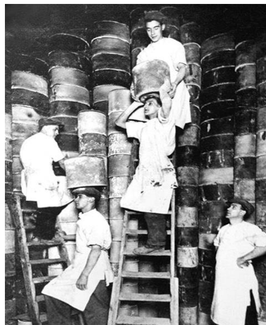
Fig.2.29 A team of Placers at work within a firing chamber. Note the clay gasket wad between the saggars. This technique is only used within a glost (glazing) oven Image courtesy Mrs L. Spencer
