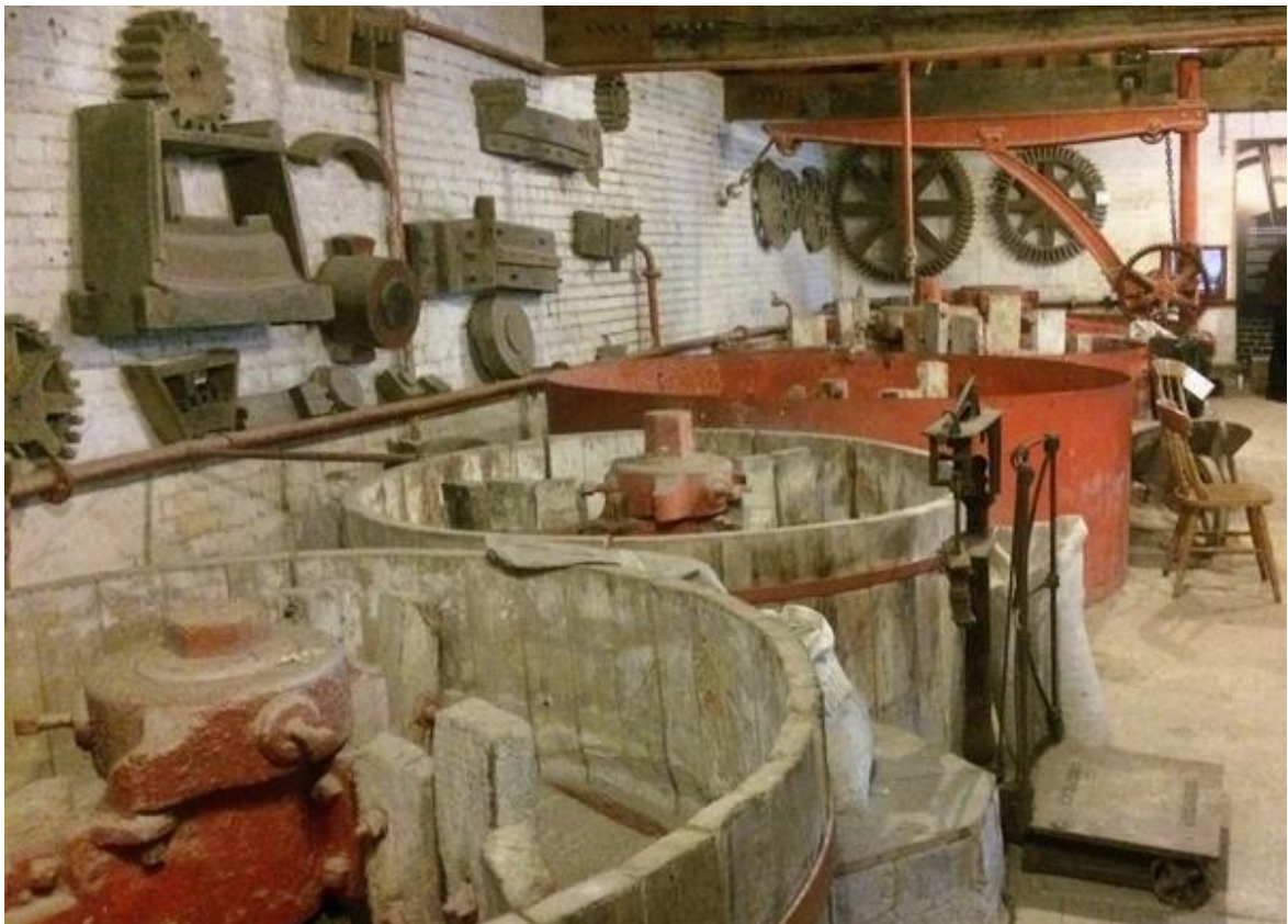
Fig.8.15 Shirley's Mill tub grinders on floor above the bevel gears *
