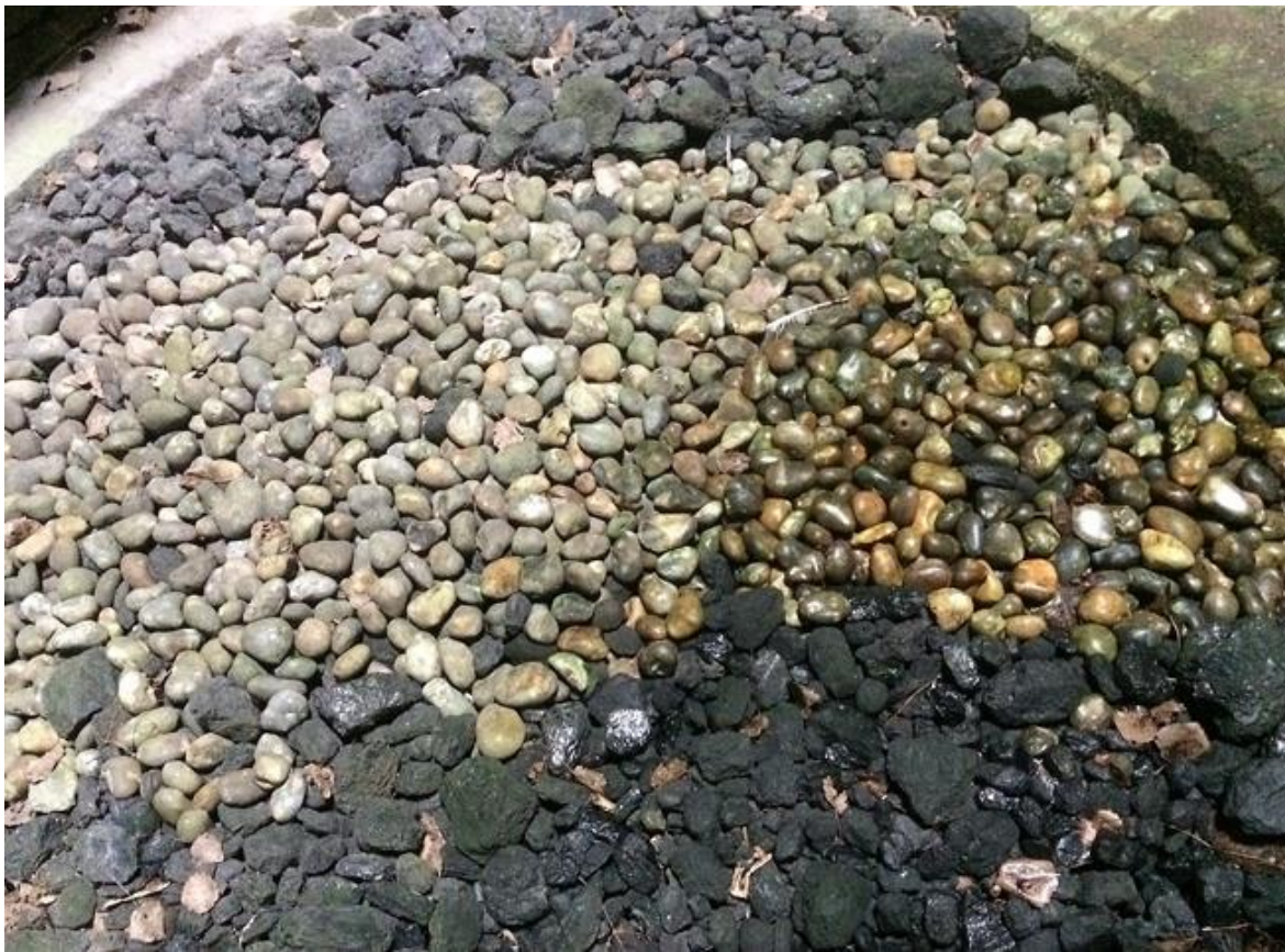
Fig.8.13 Shirley's Mill calcining kiln filled with flints (chert) and coal ready for firing *
